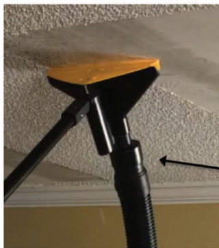
Figure 3: Preferred Hose Configuration
